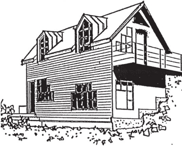
(3.7.2) Vary the mass of a building to reduce the bulkiness, including stepping a building foundation.
