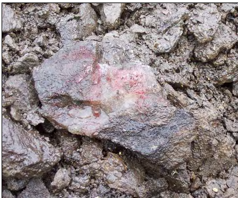
Figure 45. When alpha, alpha-dipyridyl is applied to a soil containing reduced iron, a positive reaction is indicated by a pink or red coloration to the treated area.
