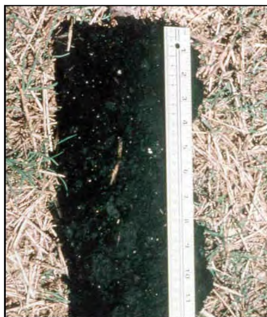
Figure 7. Black organic surface layer greater than 11 in. (28 cm) thick.
