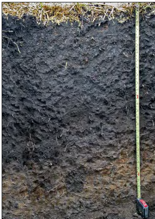
Figure 9. Deep observations may be necessary to identify the depleted or gleyed matrix below a thick, dark surface layer. In this example, the depleted matrix starts at 20 in. (50 cm).
