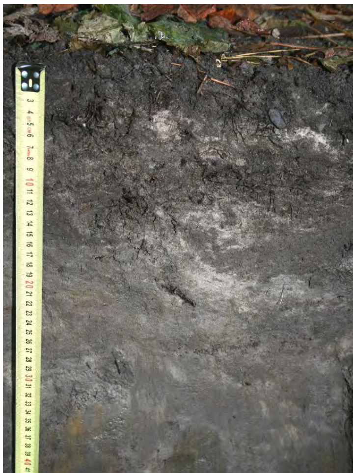
Figure 19. Redox depletions (lighter colored areas) are scattered within the darker matrix. Scale is in centimeters.
