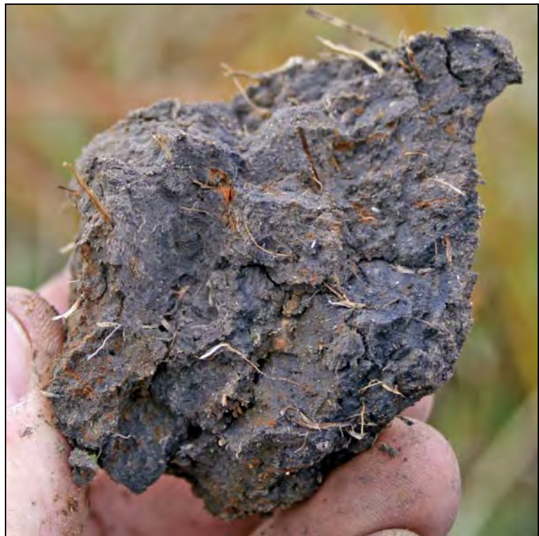
Figure 18. Redox features can be small and difficult to see within a dark soil layer.
