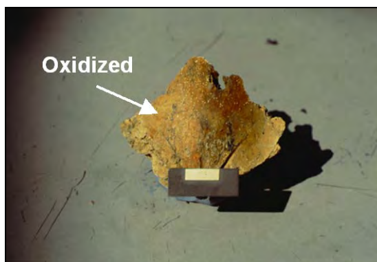
Figure 56. The same soil as in Figure 55 after exposure to the air and oxidation has occurred.
