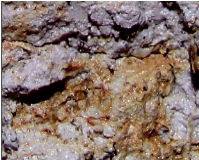
Figure 24. Water glistens on the surface of a saturated soil sample.
