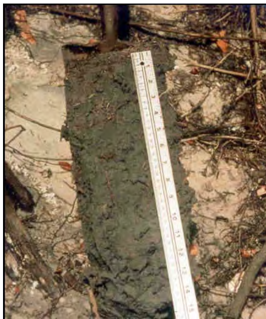
Figure 11. In this example, the gleyed matrix begins at the soil surface.
