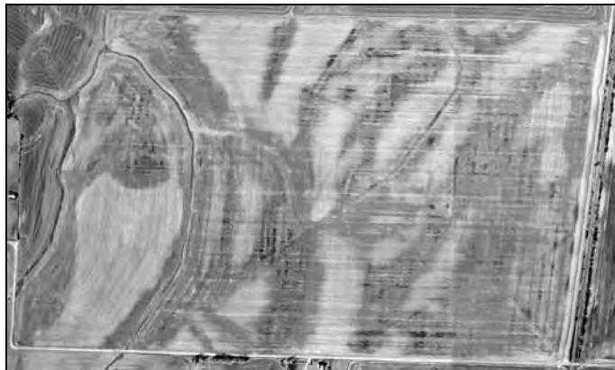
Figure 47. Aerial photograph of an agricultural field with saturated soils indicated by darker colors.
