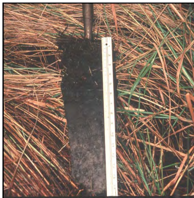
Figure 10. The mucky modified sandy layer is approximately 3 in. (7.5 cm) thick. Scale in inches on the right side of ruler.
