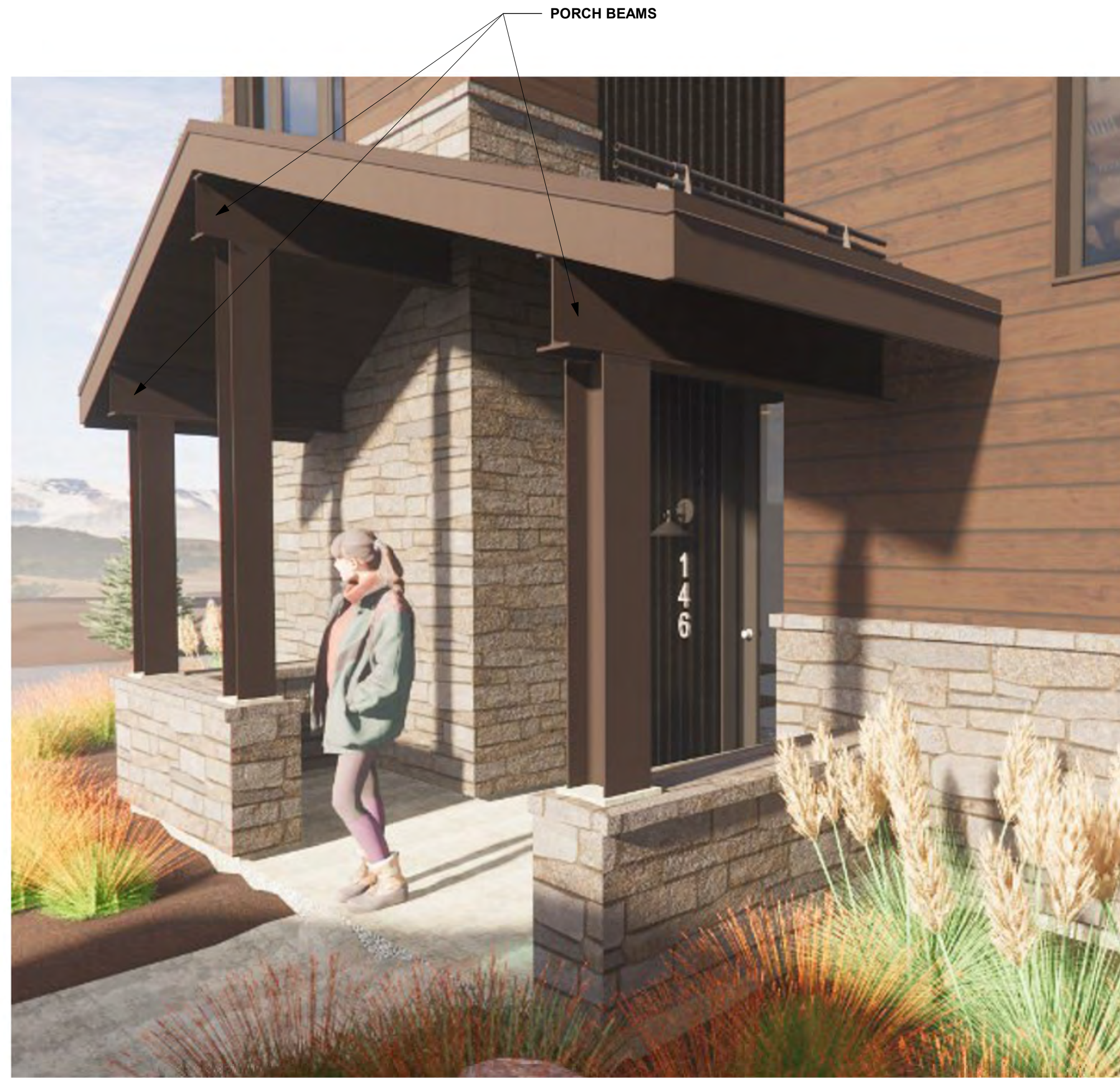
PERSPECTIVE TO DEMONSTRATE SCALE OF PORCH ROOF BEAMS WHICH ARE NOT AS APPARENT IN THE ORTHOGONAL ELEVATION
