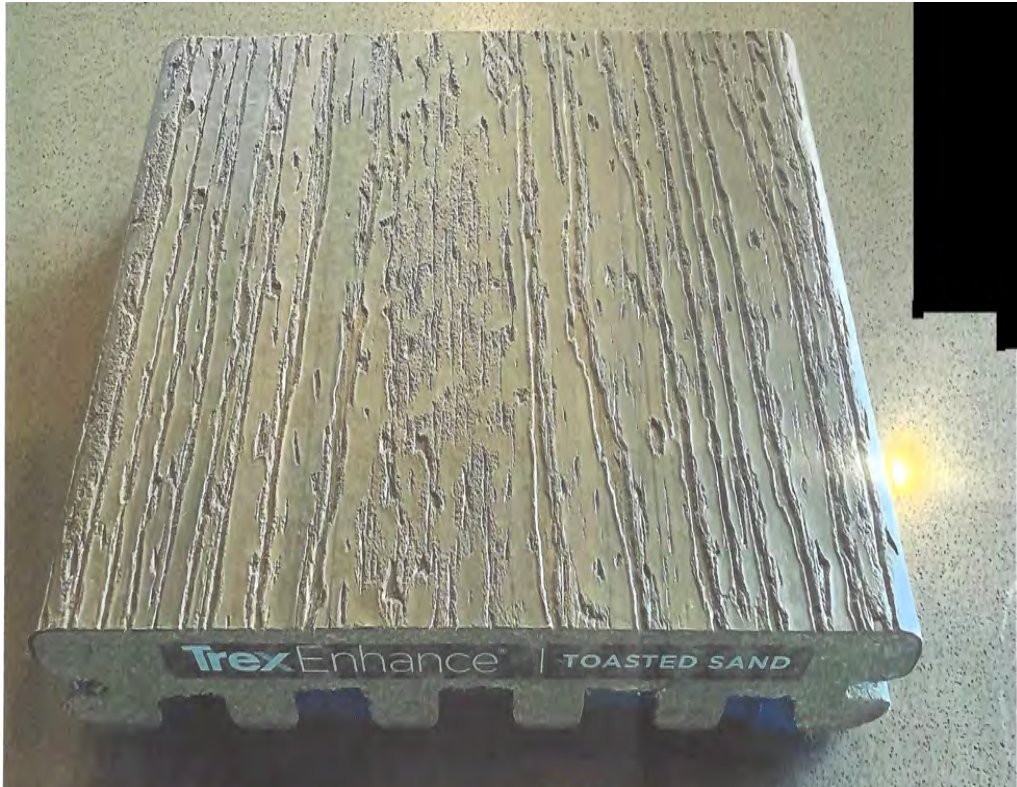
Decking Material: TREX Enhance -Toasted Sand
