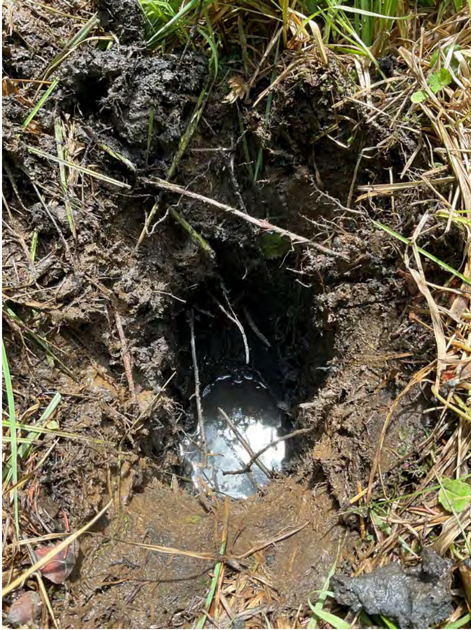
Photograph 6. View of soil pit in wetland, A16-W1, with Histic Epipedon hydric soil indicator, and saturation to surface.
